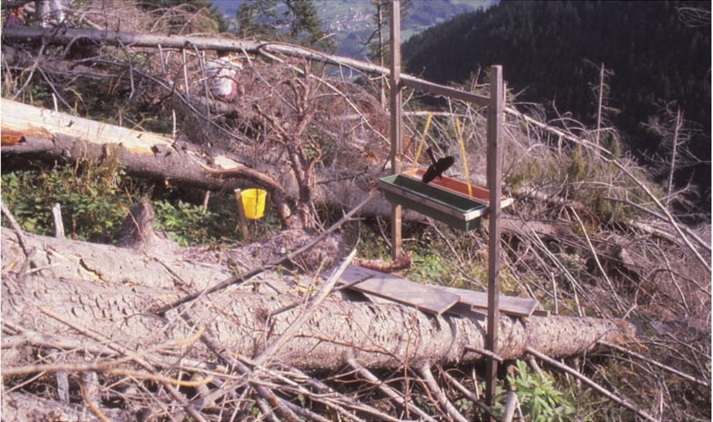
**Figure 2.** Window flight interception trap with water tray below glass screen and yellow pan trap in an uncleared Vivian windthrow (ID) plot in the Alps (Schwanden, Canton Glarus, Switzerland). Second year after the storm. Photo: © WSL (1992)
